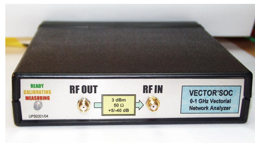
Figure 1: VECTOR'SoC: 1 GHz Vectorial Network Analyzer
